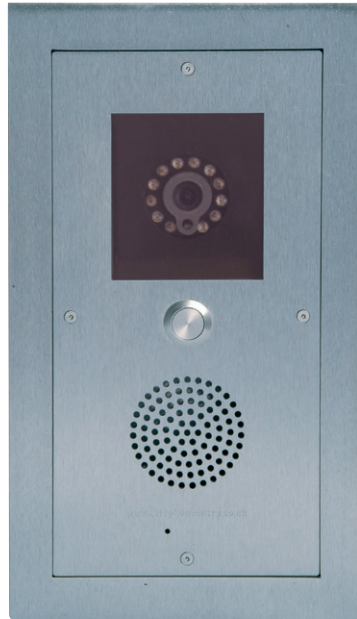
VF1-HM flush flanged BS316 grade s.steel anti-vandal telephony audio panel with day/night (colour/mono) camera.
