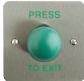
EX-MUSH-F Exit button "Mushroom" type, flush mount s.steel internal. Max distance from door handle = 1m. Max height AFFL = 1m.
