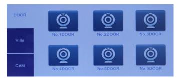
Panels & IP Cameras – monitoring all Panels and IP Cameras setup to the system from IPVIEW Monitor Interface. Can trigger Unlock function and take real time snapshot saved into the internal or external (MicroSD card)
