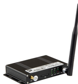
IGSM4G/IP router modem Only required if 4G aerial needs to go on roof, max 80 metres from IPGUARD (usually in top floor riser), MD-ANT345G and AR122 PSU included.
