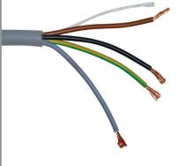
CABLE REFERENCE: 4 x 1 YY/LSZH PER LOCK Fail safe locking relies on the locking receiving the correct voltage and current. Fail secure electro-mechanical locking always requires a 3rd core control cable. Only industry reference 4 x 1 YY/LSZH cabling (or Fire Protected equivalent, if applicable) is to be used. Alarm, data or communications cabling; for example; CAT5E, CW1308 is unacceptable.
