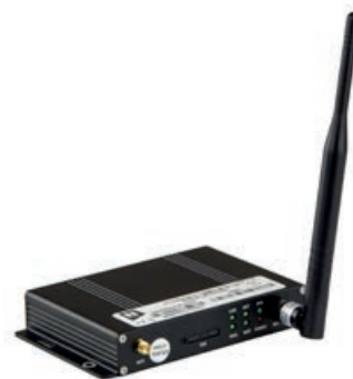
IGSM4G/IP router modem Only required if 4G aerial needs to go on roof, max 80 metres from IPGUARD (usually in top floor riser), MD-ANT345G and AR122 PSU included.
